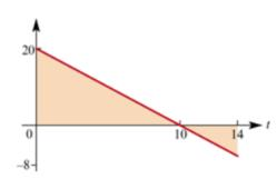
It slows for the first ten seconds. At time t=10, it is 100 m to the right of its starting point. It then heads to the right for 4 seconds. When t=14 it is 84 m from its starting point.
